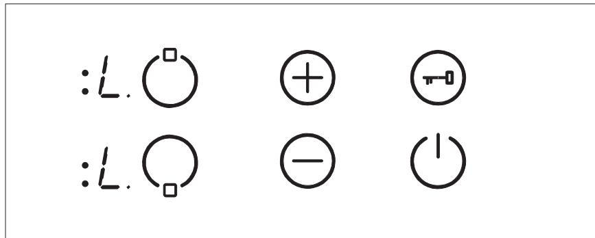
In the case the minute minder is still running, it will proceed until '00' is reached and the timer will beep. After confirmation of timer run out, the appliance is fully locked. None of the buttons can be used as long as the appliance is locked.
