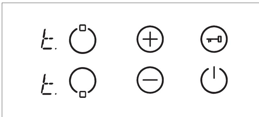
After the temperature falling, the 't' displays will be erased and the hob control unit falls back into the S-Mode. This means that the user can reactivate the appliance by touching .
