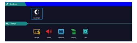
Press the  $\square$  menu  $\square$  button to display the menu, press the up and down keys to select the appropriate settings, press the right button to enter the relevant settings.
