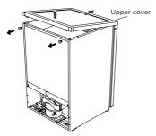
Dismantle the upper cover, fitting screws of upper hinge, and remove the upper hinge, please keep the door vertical in whole process for avoiding falling down.
