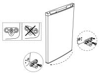
**6.** Put the door on bottom hinge and assemble the upper hinge, screws.
