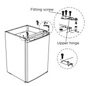
Dismantle the door and the bottom hinge assembly and adjustable foot, then assemble the bottom hinge assembly and adjustable foot on other side.
