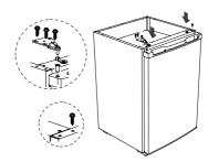
Change the cover blade on the upper cover from the left to the right. fix top cover of refrigerator.
