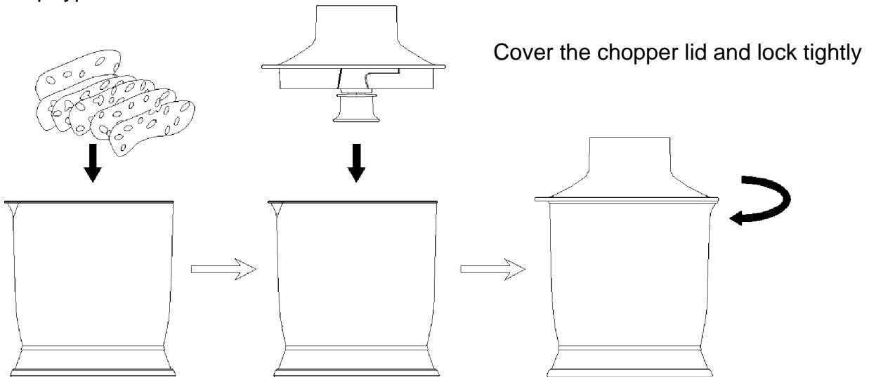
③ Let the main unit turn-lock clasp to the chopper lid, and then plug in and press the switch button. Once the food material chopped to your expected effect, just release the switch button, and the product will stop working. Finally, you should unplug the power cord firstly and then pour out the processed food.
