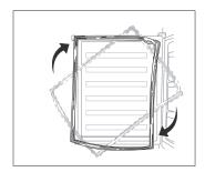
8. Place the door back on. Ensure the door is aligned horizontally and vertically, so that the seals are closed on all sides before finally tightening the top hinge.
