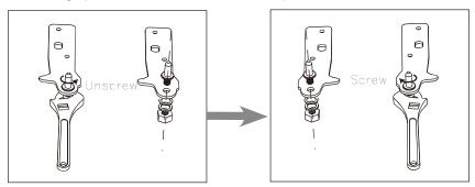
6. Refit the bracket fitting the bottom hinge pin. Replace both adjustable feet.
