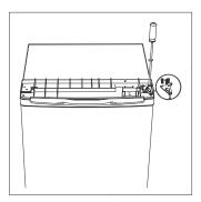
4. Unscrew bottom hinge. Then remove the adjustable feet from both sides.
