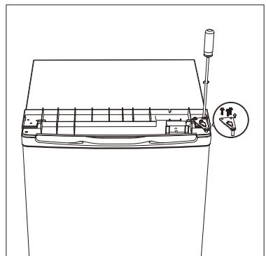
4. Unscrew bottom hinge of freezer door. Then remove the door and place it on a soft pad to avoid scratch.
