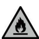
**! WARNING!** During using, service and disposal the appliance please pay attention to symbol similar as left side, which is located on rear of appliance (rear panel or compressor) and with yellow or orange color.
