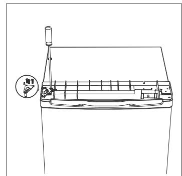
9. Put the top cover and fix it with 2 screws on the back.
