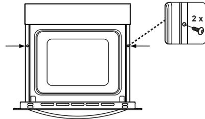
Insert the oven into the cabinet by pushing it forward. Open the oven door and insert 2 screws in the holes located on the oven frame. When the product frame touches the wooden surface of cabinet, tighten the screws.
