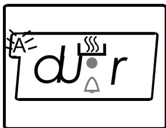
This function is used to cook after a certain period of time, within a certain duration. The food to be cooked is put into the oven. The oven is adjusted to the desired cooking function. The oven thermostat is adjusted to the desired degree depending on the dish to be cooked.
