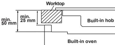
If the oven is installed under a hob, the distance between the worktop and the top panel of the oven must be a minimum of 50 mm and the distance between the worktop and the top of control panel must be a minimum of 25 mm.
